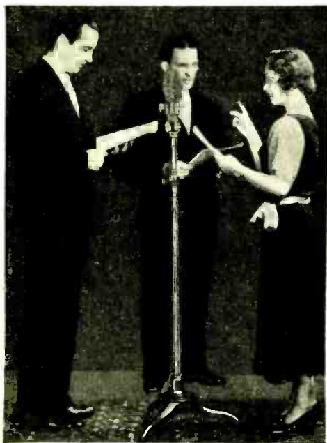
Fig. B An illustration of the flexibility possible in placing the artists with the new microphone. In the older types, it was necessary for all the artists to face the front of the microphone, but with the Velocity microphone, the artists may be anywhere around it.
